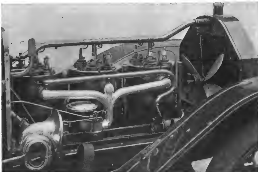
INLET SIDE OF MOTOR OF THE GREAT CHADWICK SIX.
